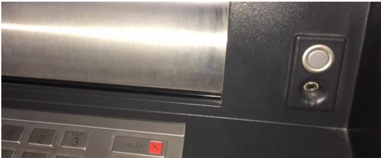
*Figure 2. The audio input jack is located above and to the right of the keypad.*
